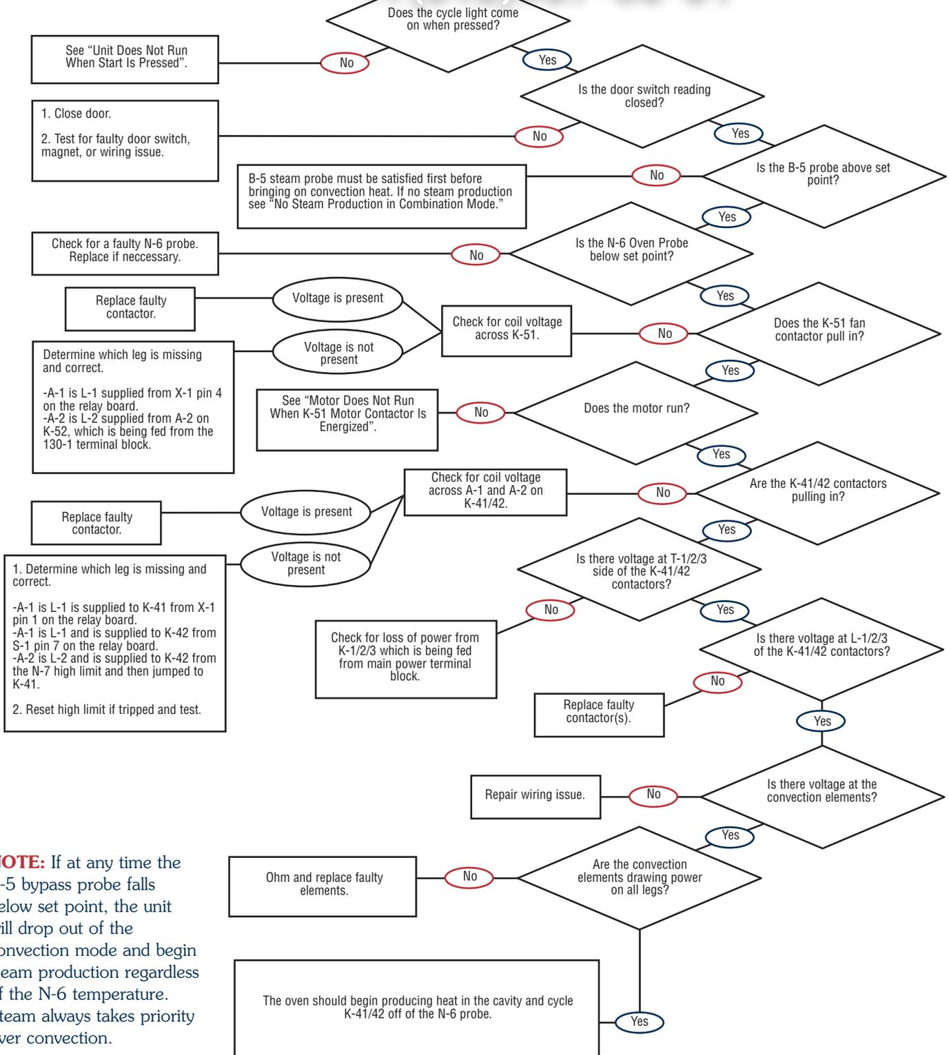
**NOTE:** If at any time the B-5 bypass probe falls below set point, the unit will drop out of the convection mode and begin steam production regardless of the N-6 temperature. Steam always takes priority over convection.
