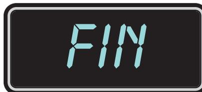
At the end of the cleaning cycle “FIN” will appear in the display. Turn the **Cooking Mode** dial to the **OFF** position.
