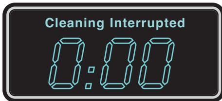
Press the start/stop key to return the oven to normal operation.
