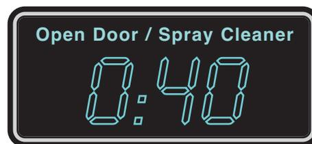
Wearing safety glasses and rubber gloves, open door, remove the drain screen and spray Combitherm liquid oven cleaner directly into the drain pipe.
