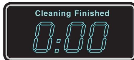
At the end of the cleaning cycle, the oven will beep and the display will indicate the end of the cycle.
