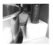
2. Place the bowl onto the mixer making sure that the holes on each side are securely placed over the pins on the bowl support. Secure the bowl by pushing the bowl clamps on either side back so that the clamps rests on the bowl handles.
