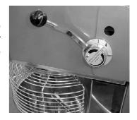
7. When the ingredients have been thouroughly mixed, press the stop button. Lower the bowl by pushing the bowl lift lever back and down to its resting position. Rotate the bowl guard so that it is in the open position. Rotate the tools anticlockwise for unhooking it and use levers to take the bowl with the tool out.
