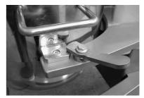
3. Rotate the bowl guard so that it rests in the open position and lower the bowl in its resting position. Select the appropriate tool and insert it onto the tool shaft rotating the tool clockwise. Insert the entrainment pin as shown in the figure. Low and insert the tool blocking ring.
