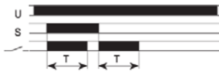
FZ12: Signal ON and OFF delay
