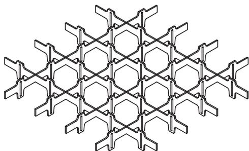
COD. 10308 SEPARATORE A 9 SCOMPARTI PER TELAIO 50mm
