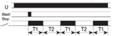
FZ40: Symmetrical recycling, OFF start with Start/Stop pushbutton
