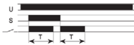
FZ12: Signal ON and OFF delay
