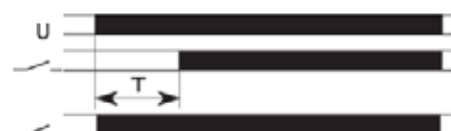
FZ16: ON Delay (1 timed contact + 1 instantaneous contact)
