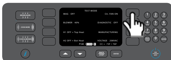
Figure 23: Test Mode: EC Fan Test
