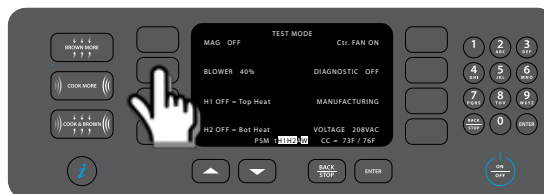
Figure 19: Test Mode: Blower Test
