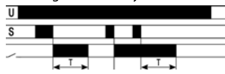
FZ81: Signal OFF delay
