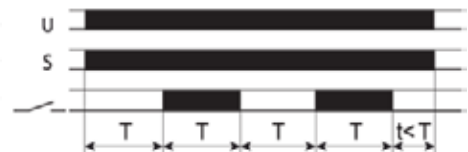
FZ31: Symmetrical recycling, OFF start, with signal contact
