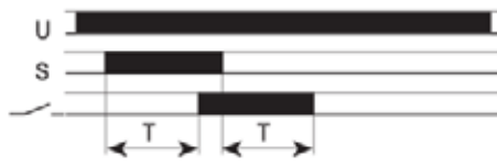
FZ16: ON Delay (1 timed contact + 1 instantaneous contact)
